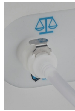
c. Correct connection – it should 'click' into place
